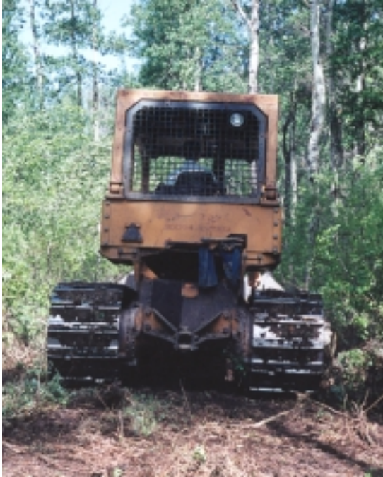
Fig. 4.6. Conventional seismic operations in Alberta involve the creation of long linear access corridors using bulldozers. (Photos: R. Schneider, left; C. Wallis, right)
