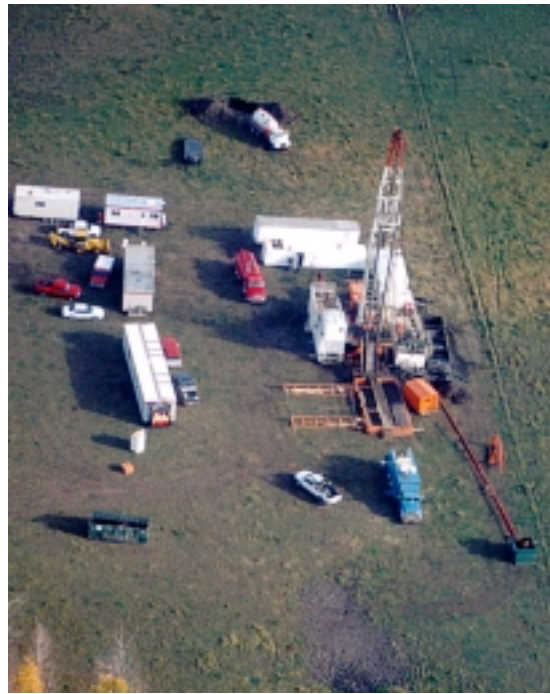
Fig. 4.8. Conventional oil drilling rig and support equipment. (Photo: Al-Pac)
