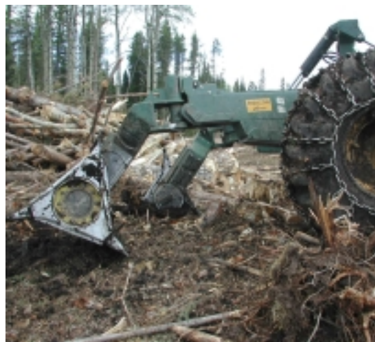
Fig. 3.7. Mound scarifier, used in preparing ground prior to planting conifers. (Photo: D. Mussell)
